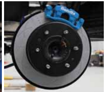
BENDIX ULTIMATE 4WD™ BIG BRAKE UPGRADE KIT Rear Disc Brake Rotor & Caliper
