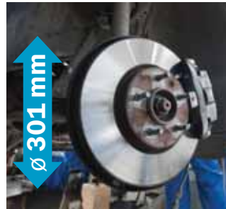
OE Disc Brake Rotor & Caliper
